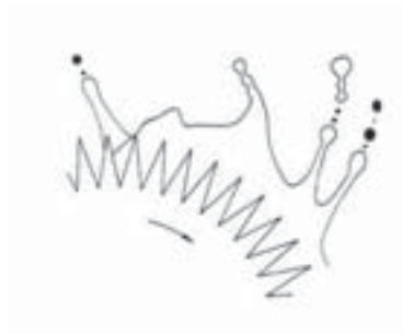
Sheet formation (breakdown of controlled droplet application)
