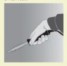
Excessive bending of the wrist is required to use this tool.
