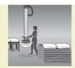
A vacuum operated lifting device can reduce the forces, awkward postures, and movements required to manually load products onto pallets.
