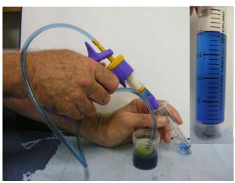
The vaccinator can be calibrated before use, by injecting a number of doses of cooled boiled water through the syringe into a measuring device. In this case, 10 doses of 2 ml should equal a total of 20 ml. We have used a 20 ml syringe barrel with the tip blocked with BluTack. Other small accurate measuring cylinders are also useful. The blue water is just to show up in the photo!
