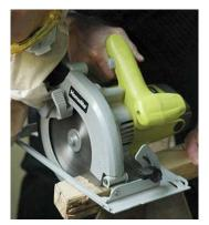
4. Be sure the lower blade guard returns to its position when you exit the cut.
