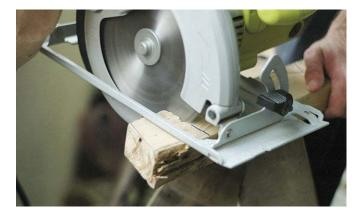
4. Push the saw into the material. Use enough force to keep the blade cutting, but avoid pushing so hard the motor speed seems to decrease, or binding occurs on the blade. A sharp blade should pass through any but the hardest materials with minimal effort.
