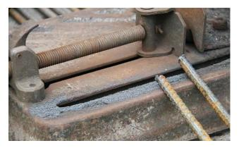
Having the working surfaces covered with residue means that your measurements may not be accurate as the metal will not lie flat.
