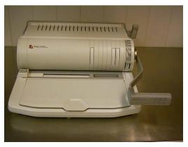
**Coil Binder**Machine used for coil binding documents.
