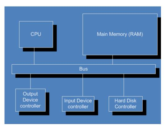
As you can see from the diagram of our imaginary PC, the CPU, the RAM, and the input and output devices can send and retrieve information in the form of electrical signals passed over buses.
